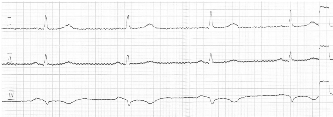
Fig. 23. Deformation of ECG curve as a result of interference of current
