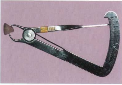
Fig 9-6 Measuring the thickness of a provisional crown.
