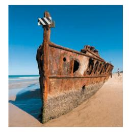
▲ Iron, although widely used as a structural and building material, corrodes easily.
