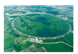
▲ The Fermi National Accelerator Laboratory has a particle accelerator 4 mi in circumference that is able to accelerate protons to energies of 1 trillion eV.
