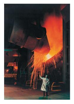
▲ Using the basic oxygen process to make steel.
