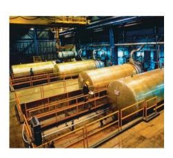
▲ Much of the uranium-235 used as a fuel in nuclear reactors is obtained by gas diffusion of UF<sub>6</sub> in these cylinders.
