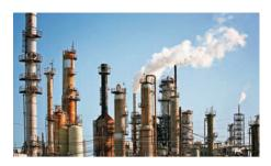
▲ Distillation of petroleum into fractions according to boiling point is carried out in the large towers of this refinery.
