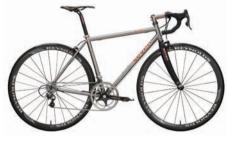
▲ This titanium bicycle doesn't corrode because of a hard, impenetrable layer of TiO<sub>2</sub> that adheres to the surface and protects the metal from further oxidation.
