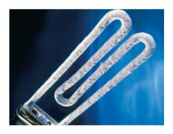
▲ Boiler scale, consisting of insoluble metal carbonates, such as CaCO₃ and MgCO₃, forms when hard water is heated.
