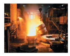
▲ Crude iron is converted to steel by oxidizing impurities with O<sub>2</sub> gas.
