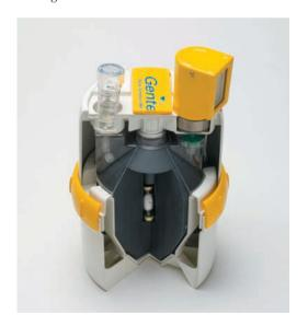
■ Technetium-99*m*, a short-lived radioisotope used for brain scans, is obtained from the decay of <sup>99</sup>Mo, which is itself prepared by neutron bombardment of <sup>98</sup>Mo and then stored in this "technetium cow" in the form of MoO<sub>4</sub><sup>2−</sup>. Small amounts of <sup>99</sup><sup>m</sup>Tc are removed by passing a saline solution through the cylinder.
