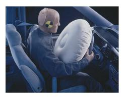
▲ Automobile air bags are inflated with N<sub>2</sub> gas produced by decomposition of sodium azide.
