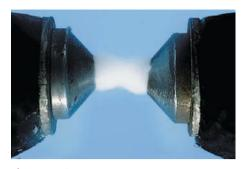
**Figure 7.16 Paramagnetism.** Why does liquid O<sub>2</sub> stick to the poles of a magnet?
