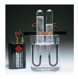
▲ Electrolysis of water gives H<sub>2</sub> gas at one electrode and O<sub>2</sub> gas at the other electrode. Which gas is at which electrode?
