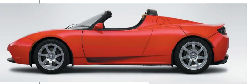
A major focus in the field of electrochemistry is the development of new and more efficient batteries. This Tesla Motors roadster, a zero-emission electric vehicle, is powered by 6831 lithium-ion batteries. It has a top speed of 125 mph, a 0-to-60 mph acceleration time of 3.9 s, and a 245 mile range.
