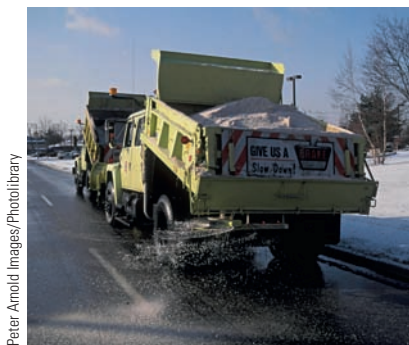
Truck applying salt, NaCl, on a snow-packed road.
