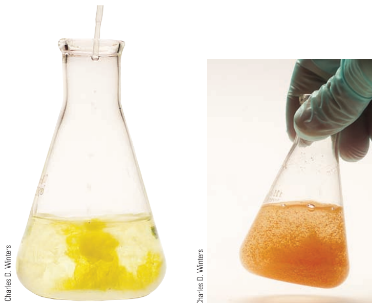
Figure 15.5 Titration of \text{Cl}^- with \text{Ag}^+ , using \text{CrO}_4^{2-} as an indicator. \text{AgCl} (cream color) comes down first, then \text{Ag}_2\text{CrO}_4 (red) precipitates.
