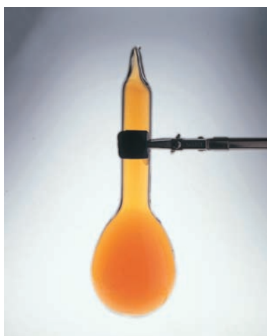
Nitrogen dioxide (NO 2 ), a binary molecular compound. It is a red-brown gas at 25°C and 1 atm.
