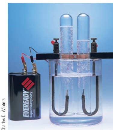
Figure 5.6 Electrolysis of water ( \text{H}_2\text{O} ). The volume of hydrogen ( \text{H}_2 ) formed in the tube at the right is twice the volume of oxygen ( \text{O}_2 ) formed in the tube at the left, in accordance with the equation 2\text{H}_2\text{O}(l) \longrightarrow 2\text{H}_2(g) + \text{O}_2(g) .
