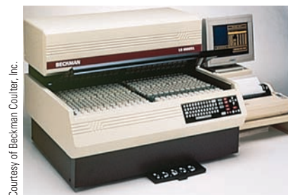
Figure 18.5 A liquid scintillation counter. This instrument is used to detect radiation and measure disintegrations per minute quickly and accurately.
