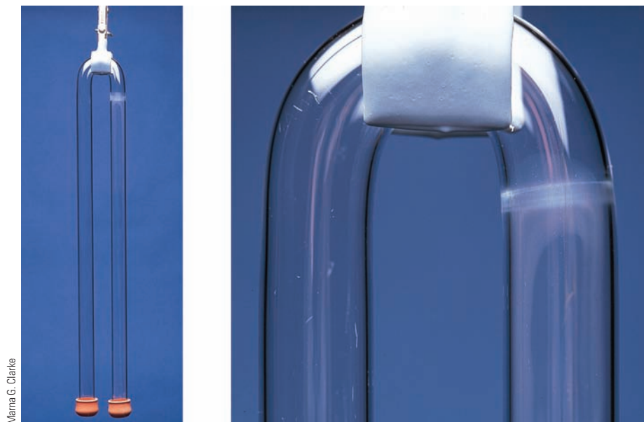
Figure 5.9 Relation of molecular speed to molar mass. When ammonia gas, which is injected into the left arm of the tube, comes in contact with hydrogen chloride, which is injected into the right arm of the tube, they react to form solid ammonium chloride: \text{NH}_3(g) + \text{HCl}(g) \longrightarrow \text{NH}_4\text{Cl}(s) . Because \text{NH}_3 (MM = 17 g/mol) moves faster than \text{HCl} (MM = 36.5 g/mol), the ammonium chloride forms closer to the \text{HCl} end of the tube.
