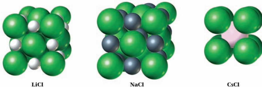
Figure 9.19 Three types of lattices in ionic crystals. In LiCl, the \text{Cl}^- ions are in contact with each other, forming a face-centered cubic lattice. In NaCl, the \text{Cl}^- ions are forced slightly apart by the larger \text{Na}^+ ions. In CsCl, the large \text{Cs}^+ ion at the center touches the \text{Cl}^- ions at each corner of the cube.
