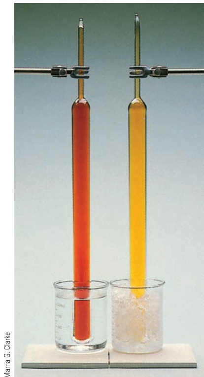
Figure 12.4 Effect of temperature on the \text{N}_2\text{O}_4\text{--NO}_2 system at equilibrium. At 0^\circ\text{C} (tube at right), \text{N}_2\text{O}_4 , which is colorless, predominates. At 50^\circ\text{C} (tube at left), some of the \text{N}_2\text{O}_4 has dissociated to give the deep brown color of \text{NO}_2 .
