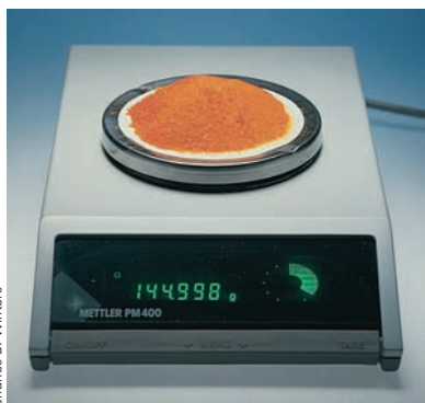
Figure 1.9 Weighing a solid. The solid sample plus the paper on which it rests weighs 144.998 g. The pictured balance is a single-pan analytical balance.
