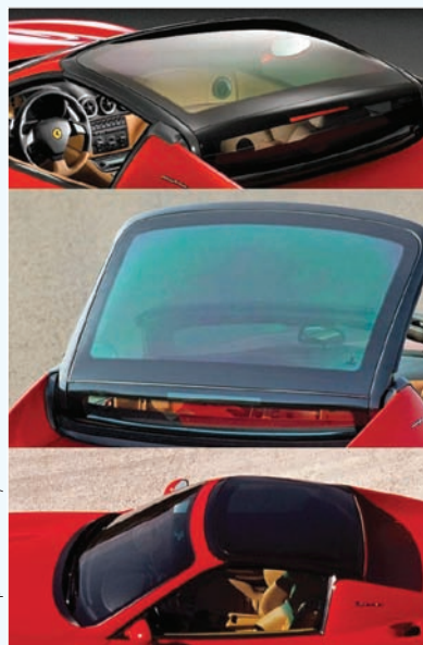
Figure A Reversible color changing electrochromic rooftop on the Ferrari Superamerica.
