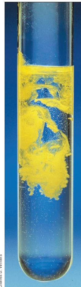
Figure 15.3 Precipitation of strontium chromate. A solution prepared by mixing solutions of \text{Sr}(\text{NO}_3)_2 and \text{K}_2\text{CrO}_4 is in equilibrium with yellow \text{SrCrO}_4(s) . In such a solution [\text{Sr}^{2+}] \times [\text{CrO}_4^{2-}] = 3.6 \times 10^{-5} .
