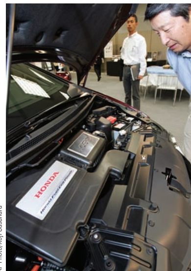
Fuel cell under Honda Clarity hood.
