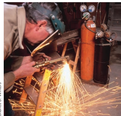
Figure 22.8 Welding with an oxy-acetylene torch.
