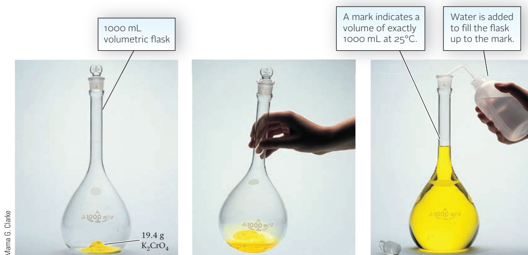
Figure 3.3 Preparing one liter of 0.100 M potassium chromate. A 0.100 M potassium chromate solution is made by adding enough water to 19.4 g of \text{K}_2\text{CrO}_4 to make one liter of solution. The weighed \text{K}_2\text{CrO}_4 (19.4 g) is transferred to a 1000-mL volumetric flask. Enough water is added to fully dissolve all of the solid by swirling. The final step is to shake the flask repeatedly until a homogeneous solution is formed.
