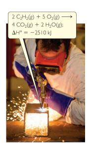
▲ Figure 22.12 Welding with an oxyacetylene torch.
