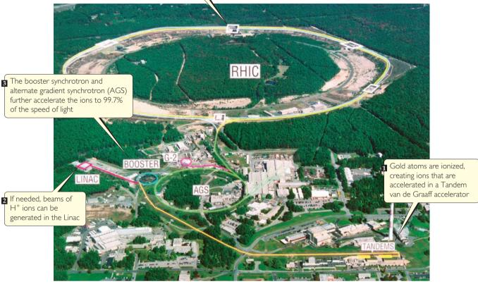
▲ Figure 21.5 The Relativistic Heavy Ion Collider. This particle accelerator is located at Brookhaven National Laboratory on Long Island, New York.
