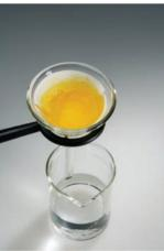
▲ Figure 1.12 Separation by filtration. A mixture of a solid and a liquid is poured through filter paper. The liquid passes through the paper while the solid remains on the paper.
