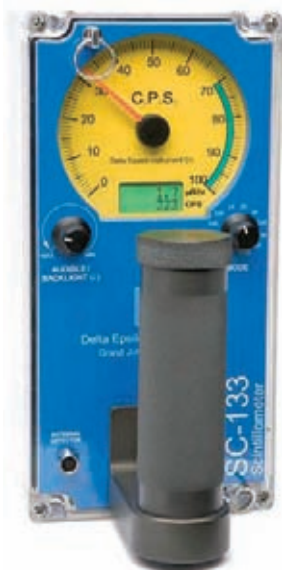
Figure 21.12 | Scintillation probe. Energy received from radiations striking the phosphor at the end of this probe is processed by the photomultiplier unit and the counts are measured on the dial. (Delta Epsilon Instruments, Inc.)
