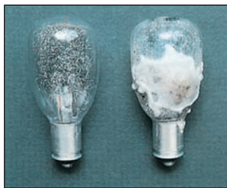
Figure 6.11 | A flashbulb, before and after firing. Fine magnesium wire in an atmosphere of oxygen fills the flashbulb at the left. After being used ( right ), the interior of the bulb is coated with a white film of magnesium oxide. (Robert Capece)
