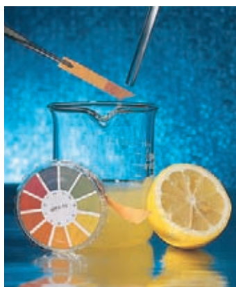
Figure 17.12 | Using a pH test paper. The color of this Hydrion test strip changed to orange when a drop of the lemon juice solution in the beaker was placed on it. According to the color code, the pH of the solution is closer to 3 than to the color for pH 5. (Andy Washnik)
