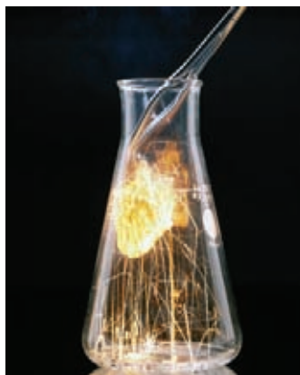
Figure 6.12 | Hot steel wool burns in oxygen. The reaction of hot steel wool with oxygen speeds up the oxidation process and the sparks and flames result. (© 1993 Richard Megna/Fundamental Photographs)
