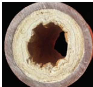
Boiler scale built up on the inside of a water pipe. (Science VU/Betz/Visuals Unlimited.)
