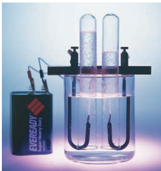
Figure 19.4 | The electrolysis of water produces \text{H}_2 and \text{O}_2 gases. It is a nonspontaneous change that only continues as long as electricity is supplied. ( Charles D. Winters/Photo Researchers )
