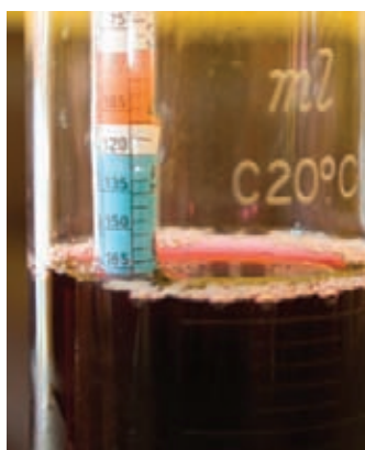
Hydrometer used for measuring sugar content in crushed grapes before fermentation. (WarrenMcConnaughie/Alamy)
