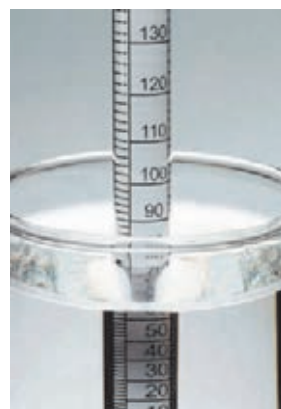
Hydrometer used for measuring alcohol content in a distilled wine sample after fermentation. (Paul Silverman/Fundamental Photographs)
