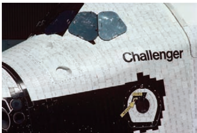
Figure 1 Space shuttle heat shield. Individual heat-shielding ceramic tiles are visible on the surface of the space shuttle Challenger . The photo was taken shortly after the spacecraft was completed. In 1986, the Challenger was lost in a tragic accident shortly after lift-off. Damage to the tiles during liftoff is believed to be responsible for the loss of the Columbia and its crew in February 2003 when the spacecraft broke apart during reentry into the earth's atmosphere. (Roger Ressmeyer/© Corbis)
