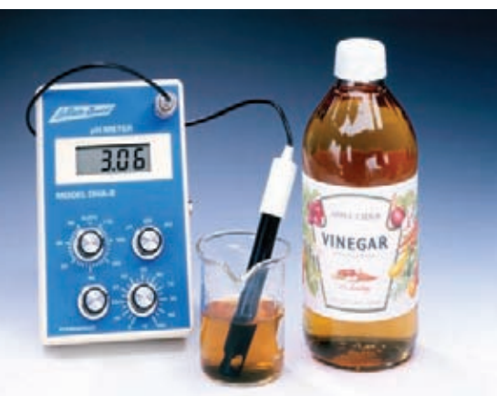
Figure 17.2 | A pH meter. After the instrument has been calibrated with a solution of a known pH, the combination electrode is dipped into the solution to be tested and the pH is read from the meter. ( Richard Megnal Fundamental Photographs. )
