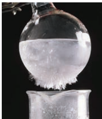
Naphthalene sublimates when heated and the vapor condenses directly to a solid when it encounters a cool surface.
