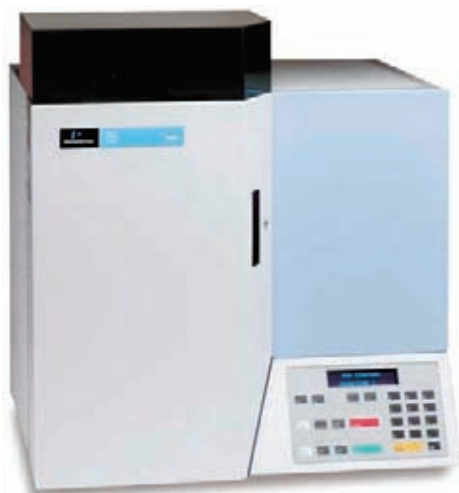
Figure 3 Elemental analysis using gas chromatography. Modern CHN analyzer. (© 2010 PerkinElmer, Inc. All rights reserved.)
