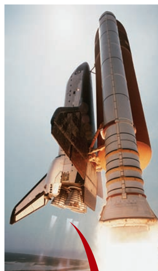
Figure 7.1 | Liquid hydrogen and oxygen serve as fuel for the space shuttle. The three almost invisible points of blue flame come from the main engines of the space shuttle, which consume hydrogen and oxygen in the formation of water. (Corbis Images)
