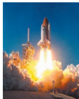
Figure 19.15 | Blastoff of the space shuttle. The large negative heat of formation of \text{Al}_2\text{O}_3 provides power to the solid-state booster rockets that lift the space shuttle from its launch pad. (NASA)
