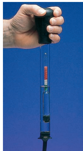
Figure 20.11 | A battery hydrometer. Battery acid is drawn into the glass tube. The depth to which the float sinks is inversely proportional to the concentration of the acid and, therefore, to the state of charge of the battery. (OPC, Inc.)
