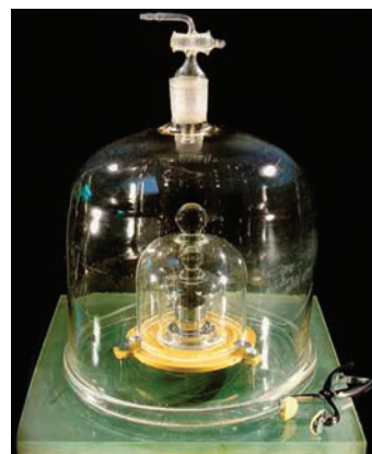
Figure 2.4 | The international standard kilogram. The SI standard for mass is made of a platinum–iridium alloy and is protected under two bell jars, as shown, at the International Bureau of Weights and Measures in France. Precise copies, called secondary standards, are maintained by many countries. (NIST)
