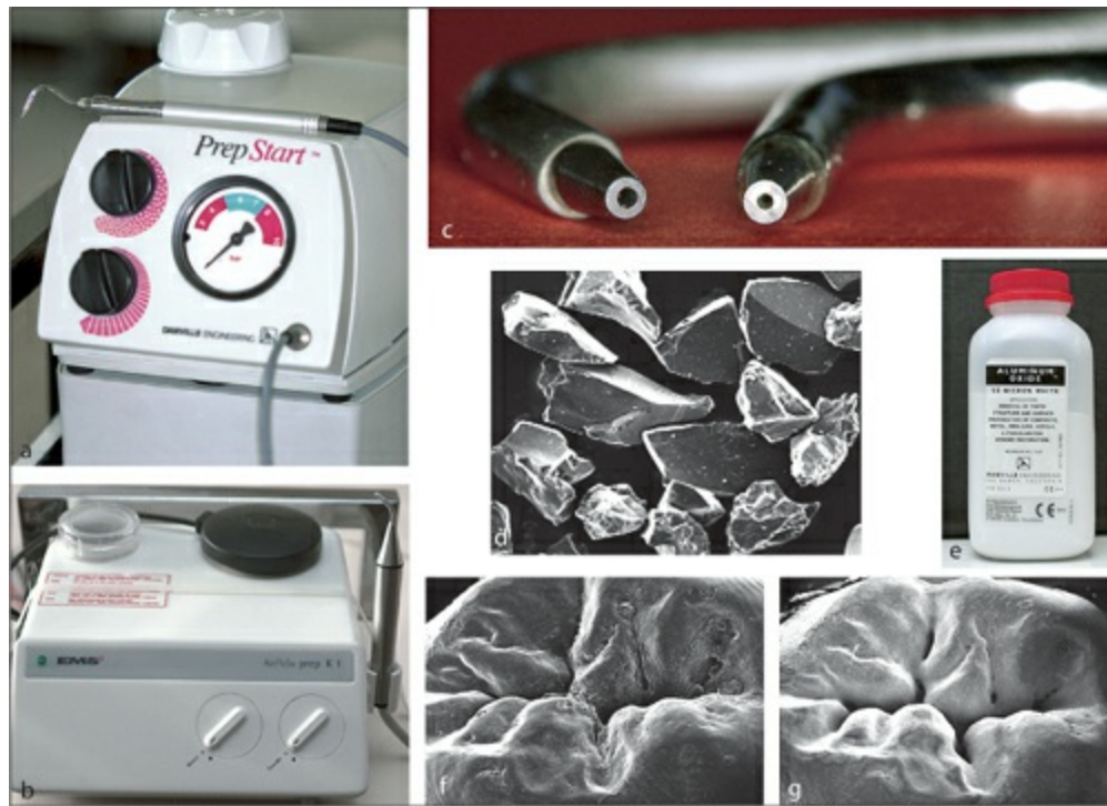
Fig 8-23 (a) PrepStart air-abrasion device (Danville Engineering). (b) Airflow Prep K1 air-abrasion device (EMS). (c) Tips of the PrepStart system with different-size spouts. The narrower the opening, the more precisely tooth structure can be removed. (d) Fe-SEM image of aluminum oxide particles (Danville Engineering) at 200× magnification. Note the irregular shape and different sizes of the particles. (e) Container of aluminum oxide particles (Danville Engineering). (f and g) Air abrasion can be used to open the occlusal fissures, thereby facilitating assessment of caries lesions (shown before and after). These minimally invasive cavities are sealed afterward.
