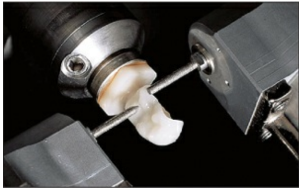
Fig 18-12 CEREC milling chamber with cylindrical diamond and tapered diamond.
