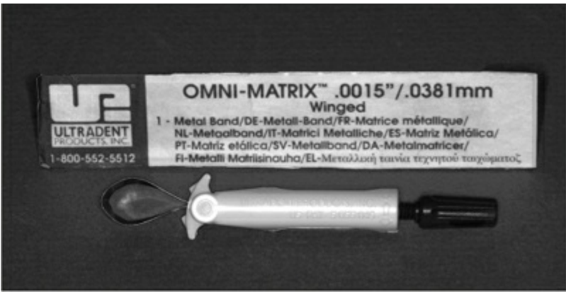
Fig 11-53 The Omni-Matrix (Ultradent) is basically a preassembled Tofflemire retainer and band that is intended for one-time use and then disposal. It is available with 0.0010- and 0.0015-inch-thick metal matrix band material, with “wings” (as shown) or without.
