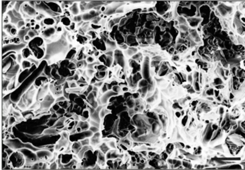
Fig 8-102 Field-emission scanning electron photomicrograph of porcelain etched with 9.6% hydrofluoric acid (Porcelain Etch, Ultradent). Bar = 5 \mu\text{m} .
